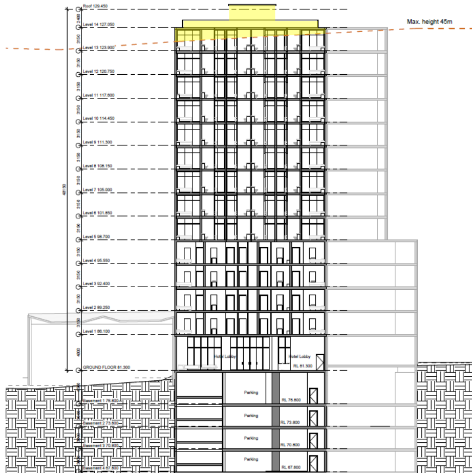
Figure 2: Section (B) showing extent of the height non-compliance (shaded yellow)
